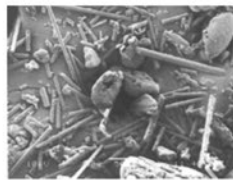
Carbon fiber (Electron microscope×300)
