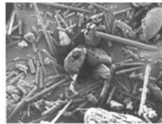
Carbon fiber (Electron microscope×300)
